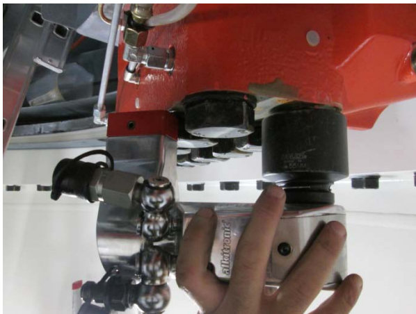
Figure 2: alkitronic® AS-3 overhead on an azimuthal brak
