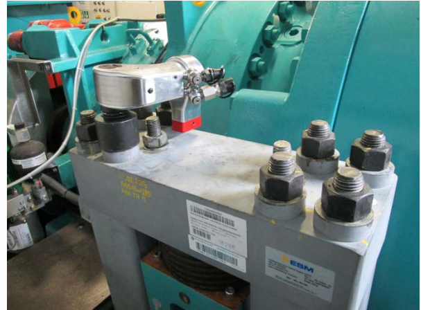
Figure 3: Hydraulic torque wrench AS-3 on pedestal bearing
