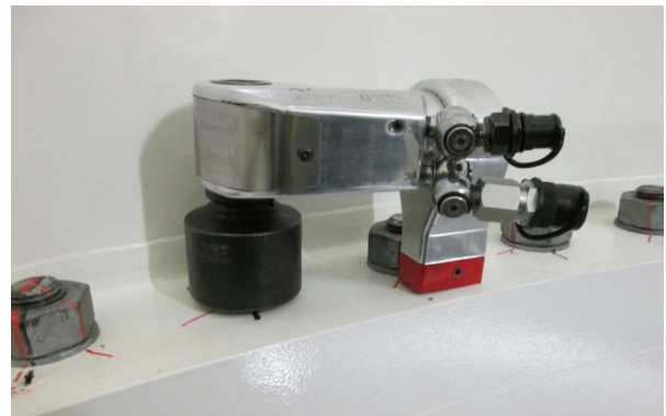
Figure 4: alkitronic® Hydraulic torque wrench AS-3 on tower flange bolts M36- high tension
