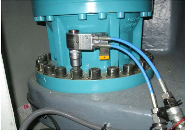
Figure 6: Hydraulic torque wrench AS-1 up to 1.100 Nm on azimuth drive
