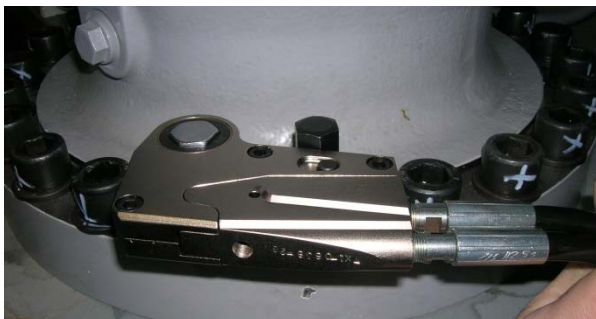
Figure 7: alkitronic® Hydraulic torque wrench AX-1 up to 750 Nm on azimuth drive
