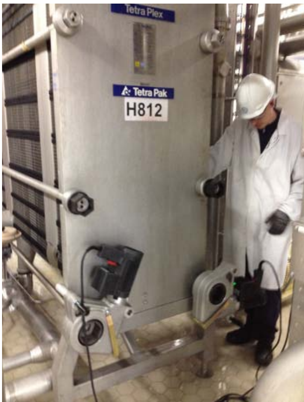
Figure 2: alkitronic radial torque multiplier in use. Photo: alki TECHNIK
