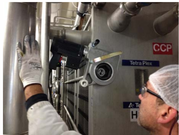
Figure 1: alkitronic torque multipliers at Tetra Pak Processing Systems B.V.; Photo alki TECHNIK
