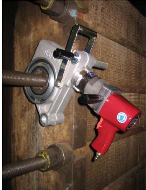
Figure 2: The alkitronic radial torque multiplier in use. Photo: alki TECHNIK
